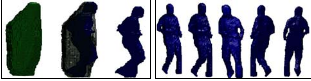
Figure 3 Results (color plates): multiple input images ref figure 1; 3D lattice and 3D reconstructed object within 3D lattice (bottom left); body model different viewpoints (bottom right)
